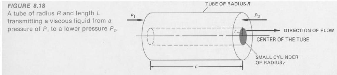
The force acting to slide this small cylinder of radius  $r$  in the direction of flow is given by the difference between the pressures acting on the ends of the cylinder times the area of the end of the cylinder,
