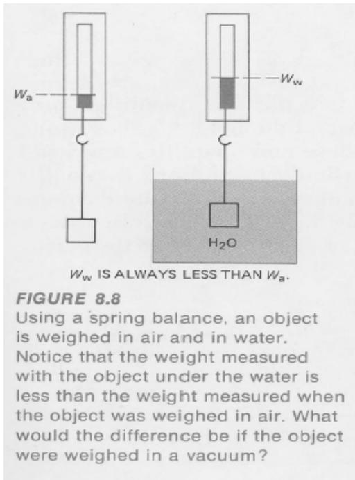
product of the density of water, the volume of the *solid*, and the acceleration of gravity.
