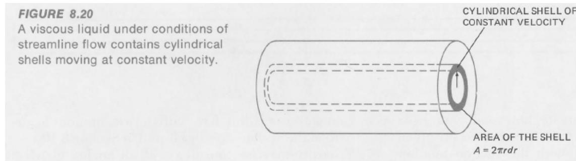
Each cylindrical shell has a different value of flow velocity as given by Equation 8.17. The area of the end of the shell of radius  $r$  is the circumference of the shell ( $2\pi r$ ) times the shell thickness ( $dr$ ),
