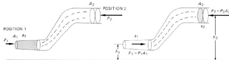
Then the surface of the liquid near position 1 will move a distance  $s_1$ . But there may exist a resisting force  $F_2$  at position 2 where the surface of the liquid will move a distance  $s_2$ . We can calculate the net work done on the liquid as we cause it to move from position 1 to 2. The net work will be given by the work we did on the liquid at position 1 minus the work done by the liquid against the resisting force at position 2,
