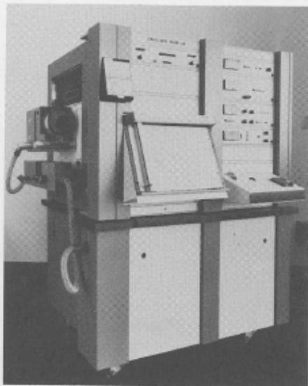
Pulmonary testing unit. The components of this basic unit are a spirometer, a CO<sub>2</sub> absorber-recorder interface, and an X-Y-T recorder. (Searle Cardio Pulmonary Group—CPI, Houston, Texas.)
