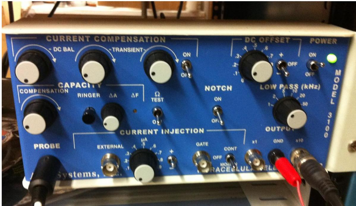
Figure 10: Front face of the intracellular amplifier used during the intracellular membrane potential recordings. The “ $\Omega$  TEST” switch used to test electrode resistance is center left. The DC offset knob is in the upper right corner, and should be turned counter clockwise to start. The ground wire is placed in the “GND” pin jack opening. The amplifier in this set-up amplifies the signal by 10X.
