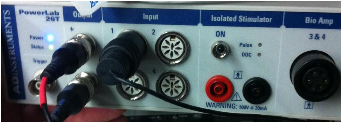
Figure 15: Power lab with BNC output and input connections from the intracellular amplifier shown.
