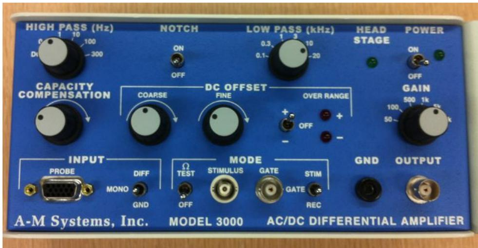
Figure 11: Extracellular amplifier used for this lab.
