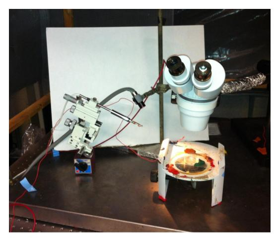
Figure 7: Placement of the preparation under the microscope with the intracellular head stage mounted on a micromanipulator
