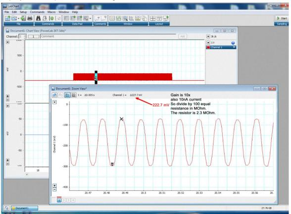
Figure 12: Traces of the responses for measuring electrode resistance.
