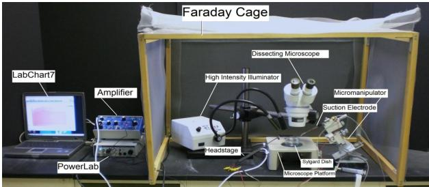
Figure 5: Overall setup of the recording equipment.
