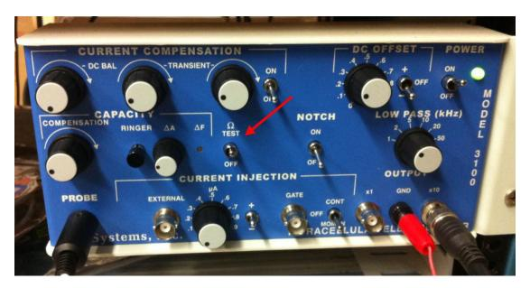
Figure 11: Front face of the intracellular amplifier with the " $\Omega$  TEST" switch in the on position.
