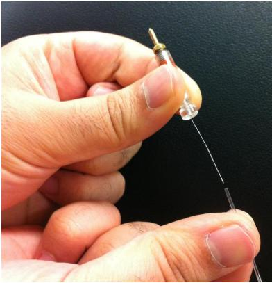
Figure 9: Microelectrode and holder
