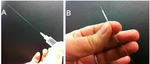
Figure 8: Filling microelectrode
