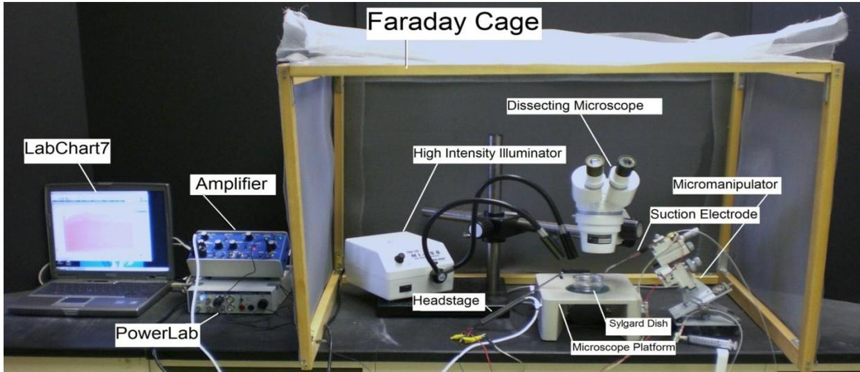
Figure 11: Overall setup of the recording equipment
