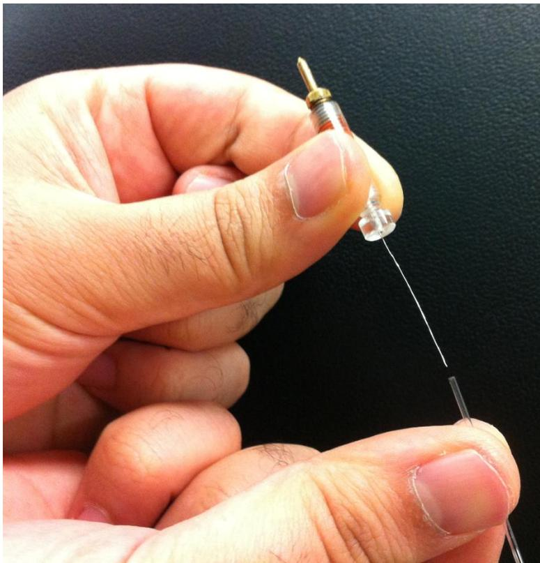
Figure 14 : Focal electrode and holder
