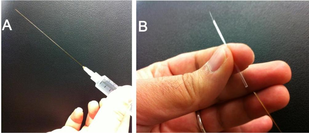
Figure 13: Filling the focal electrode with crayfish saline
