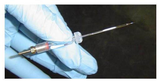
Figure 13: Microelectrode assembly with glass capillary in place.
