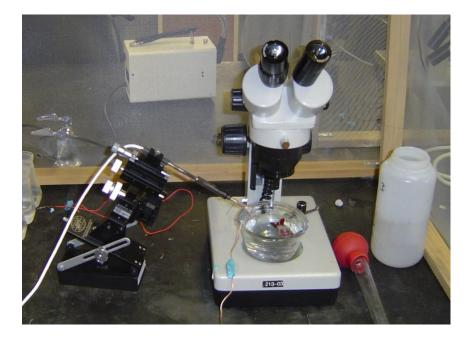
Figure 12: Placement of the preparation under the microscope. Use poster tack (shown in blue) to secure the specimen dish and ground wire to the stage of the dissecting scope.
