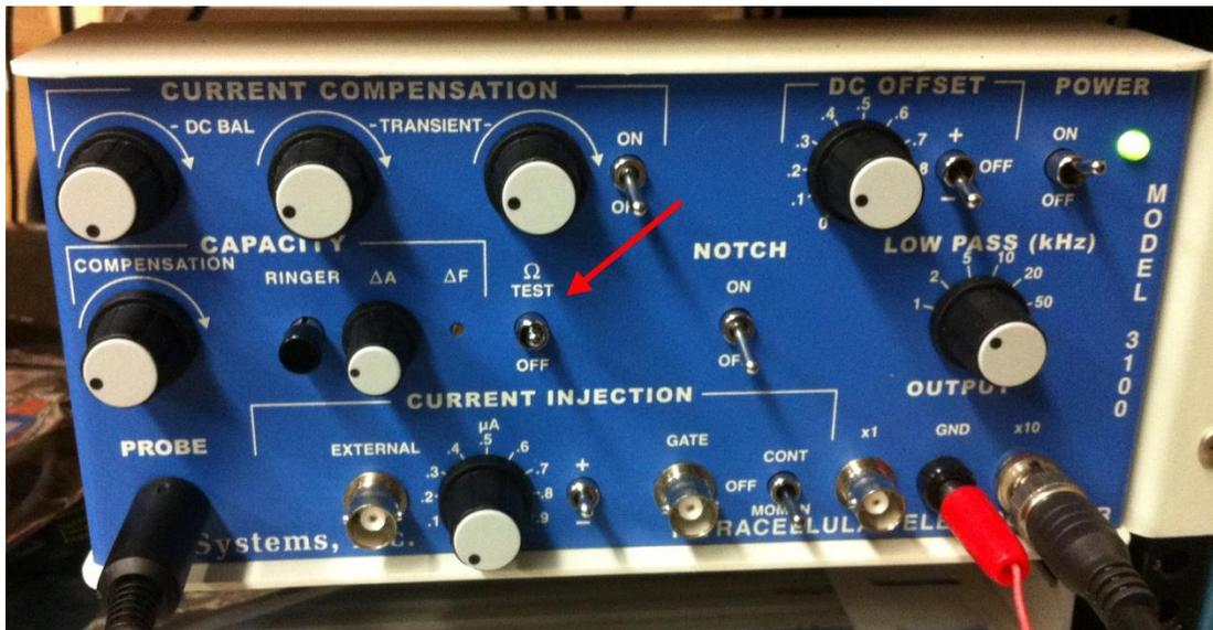
Figure 16: Front face of the intracellular amplifier with the “ $\Omega$  TEST” switch in the on position.
