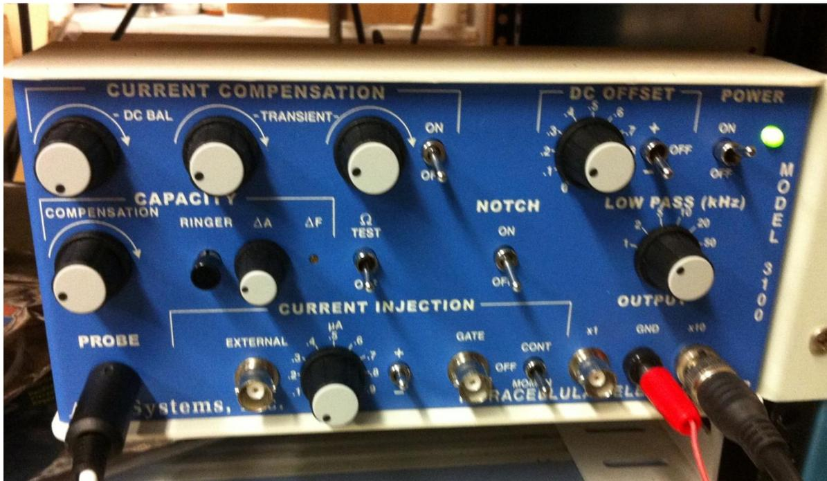
Figure 15: Front face of the intracellular amplifier used during the intracellular membrane potential recordings. The “Ω TEST” switch used to test electrode resistance is center left. The DC offset knob is in the upper right corner, and should be turned counter clockwise to start. The ground wire is placed in the “GND” pin jack opening. The amplifier in this set-up amplifies the signal by 10X.
