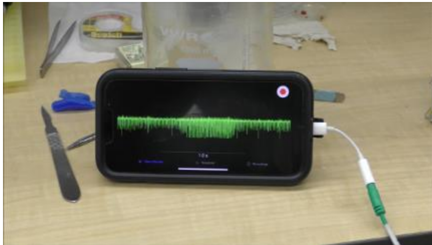
Figure 15: The Backyard brains IPHONE or IPAD AP “Spike Recorder” is used to monitor the activity. Newer IPHONES need an lighting wire adaptor to connect to the cables provided by Backyard brains.
