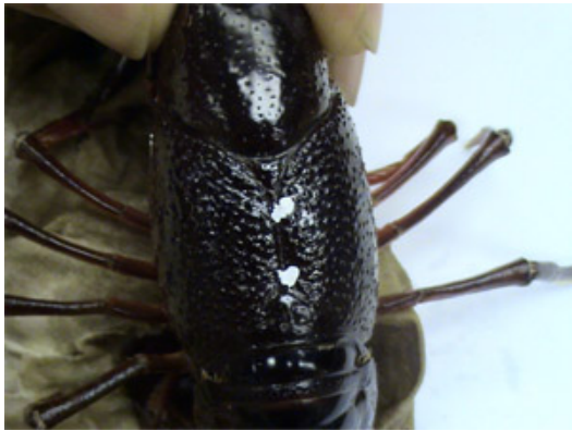
Figure 3. Placement of stainless steel wires in the thoracic chamber. The white dots on the carapace represent points for the stainless steel wires to be placed under the cuticle. The wires span the heart in a rostral-caudal arrangement. This will allow for measures of heart contraction through dynamic impedance.
