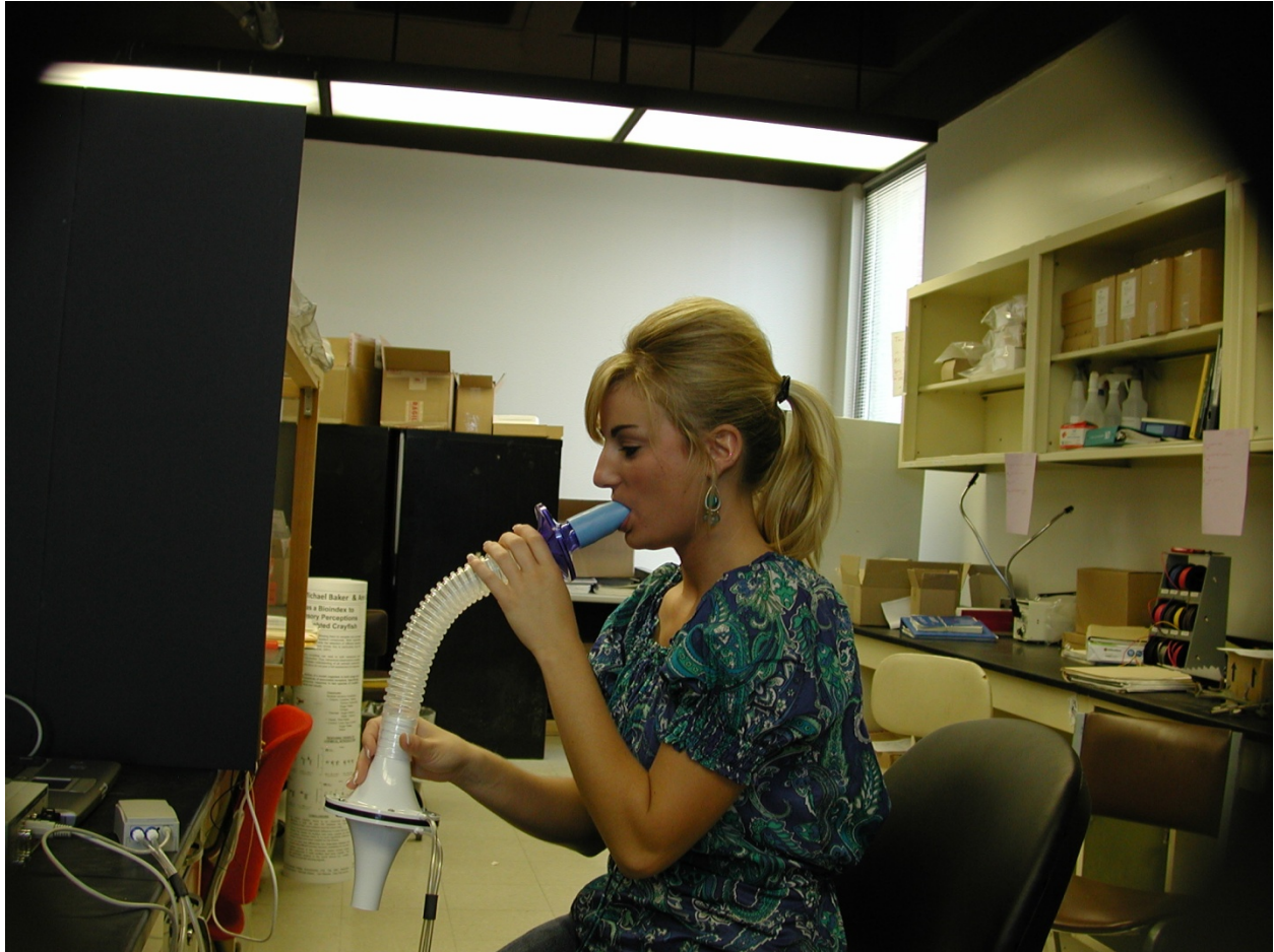
Figure 2: The image above shows the proper use of the flow head for the respiration experiment.
