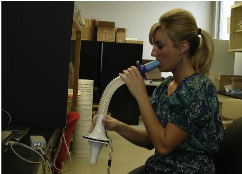
Figure 3: The image above shows the proper use of the flow head for the respiration experiment.
