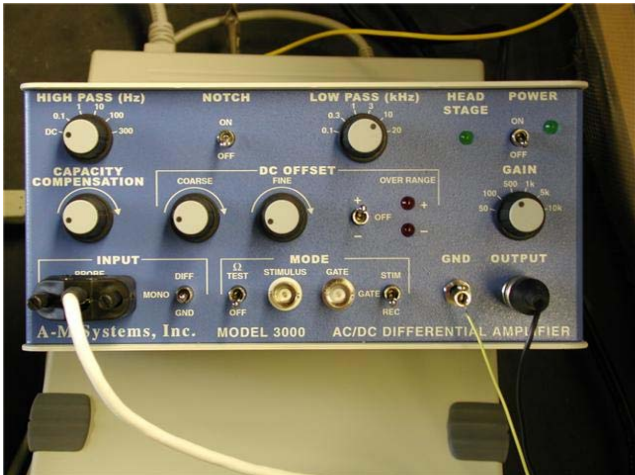
Figure 30: “Test toggle” is in the bottom row to test electrode resistance. The “coarse” knob is also found under DC offset which should be turned counter clock wise. Gain is set to 50, which amplifies signals by a factor of fifty. The ground wire from the head stage is placed in the “GND” pin jack opening.
