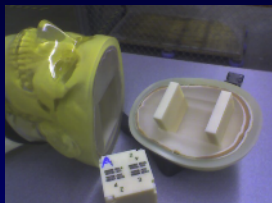
2.5" Ball Cube in cranium for fiducial and skull tracking QA
