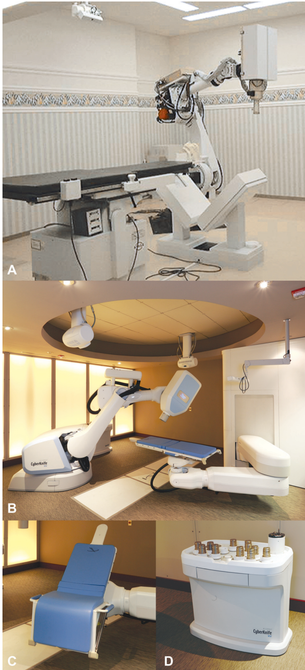
Figure 1: The CyberKnife System of (A) the late 1990's and (B-D) 2010. Panel (A) shows the first generation of stand-mounted, flat-panel image detectors (not the fluoroscopes featured in the earliest systems described in Table 1). The most obvious changes between the two systems shown are the robotic manipulator, the positions of the X-ray image detectors, the couch design, and the addition of the boom-mounted stereo camera and the Xchange Robotic Collimator Changer table. Alterations in the LINAC design are not obvious because of the covers. The couch included in (B) is the optional RoboCouch Patient Positioning System, which is shown in its seated load configuration in (C). The Xchange system table, which is obscured behind the robotic manipulator in (B), is shown in more detail in (D).
