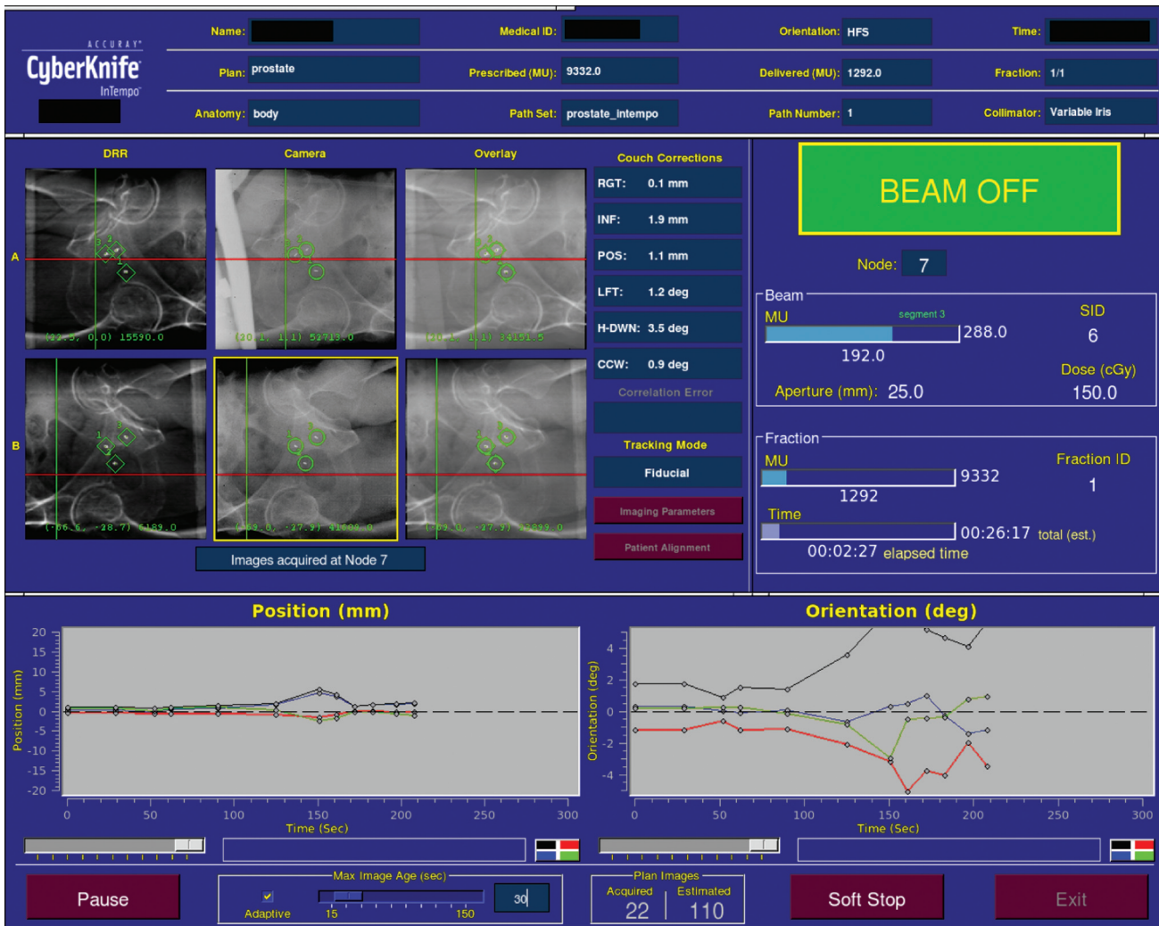
Figure 5: The treatment delivery graphical user interface (GUI) during a prostate treatment using fiducial marker tracking and the InTempo adaptive imaging algorithm. The section labeled 'couch corrections' (to the right of the X-ray images) shows the target's actual position relative to its ideal aligned position. These offsets are compensated for by realigning the beam with the target using the robotic manipulator. At the base of the screen, the history of translational (left side) and rotational (right side) corrections applied during this treatment fraction are shown. The position corrections are inferior-superior (blue), anterior-posterior (green), left-right (red), and total 3D offset (black). The rotation corrections are pitch (red), roll (blue), and yaw (green), with the sum of all angular offsets shown in black. During this treatment the first seven images are acquired with a maximum image age of 30 s. Between images 6 and 7 the prostate moves by about 3 mm, which automatically triggers the maximum image age to be reduced to 15 s, resulting in more frequent position corrections being applied (note reduced interval between images 7-12). Importantly in this case, a baseline shift in the pitch angle of 2-3° is observed during the first four minutes of treatment that would have been missed if intra-fraction corrections were not applied. With correction, this rotation is reduced to a more randomly distributed inter-correction error of about 1° on average.
