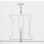
FIGURE 8.11 A spool of thread, a card, and a pin can be used to demonstrate the effects predicted by Bernoulli's equation.
