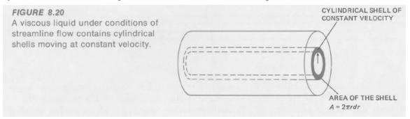
Each cylindrical shell has a different value of flow velocity as given by Equation 8.17. The area of the end of the shell of radius *r* is the circumference of the shell  $(2\pi r)$  times the shell thickness (dr),
