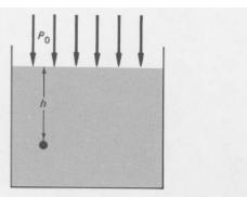
**FIGURE 8.3** A liquid in a container with a free surface, upon which a pressure  $P_0$  is acting.
