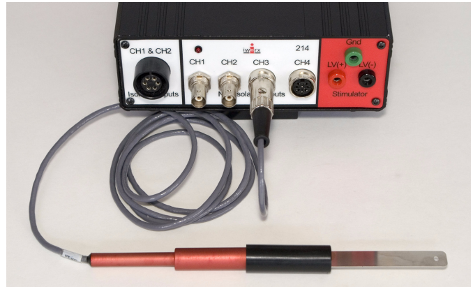
Figure AM-11-2: The FT-104 force transducer connected to an IWX/214.
